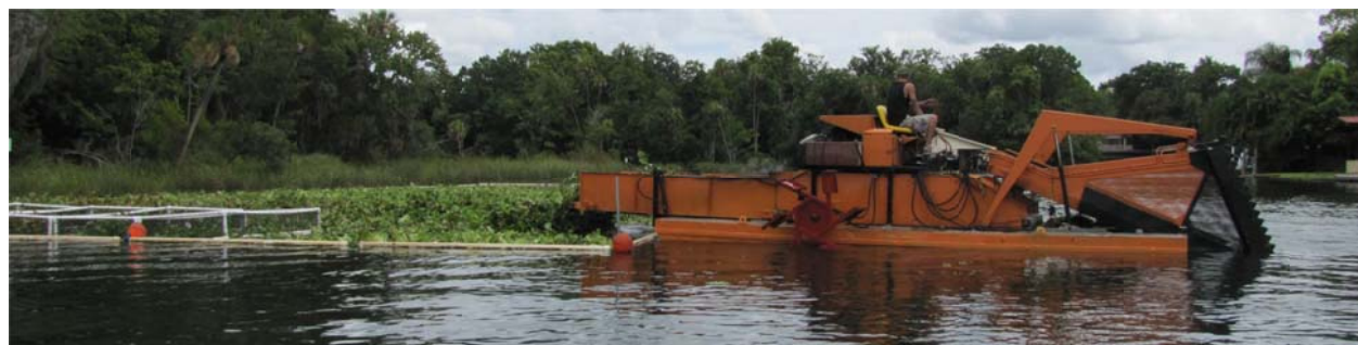
Figure 10. Use of aquatic weed harvester for water hyacinth inoculation during July 2013.
