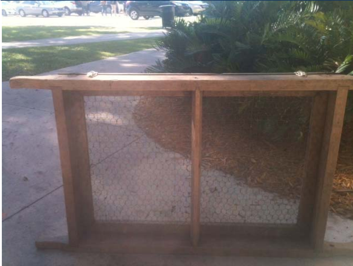
Figure 12. Hyacinth dredge used to collect fauna living in and among the floating water hyacinths.
